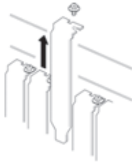
Figure 5.7 Removing an Expansion Slot Cover
