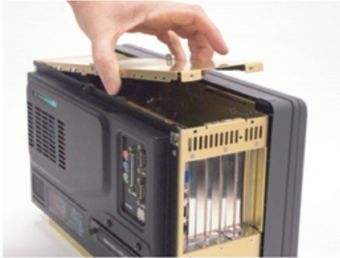
Figure 5. 5 Lift Up the Card Retention Plate
