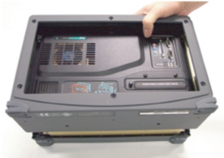
Figure 5.2 Remove the Outer Casing
