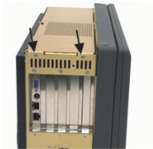
Figure 5. 4 Two Card Retention Plate Screws
