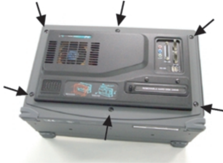
Figure 5.1 Rear Panel M4 Hex Screws (6 each)
