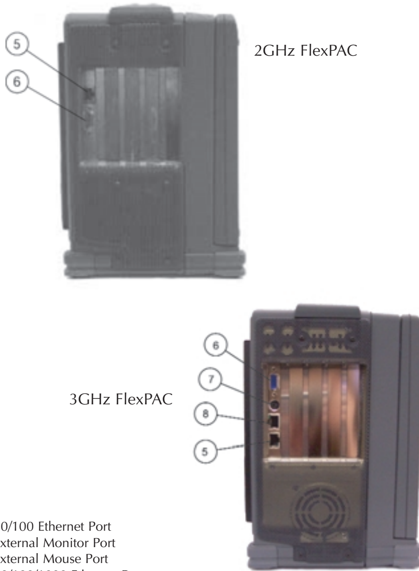
Figure 1.9 Side Panel Connections
