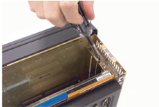
Figure 5. 6 Expansion Slot Cover - Single Screw Removal
